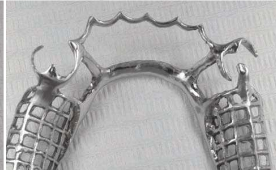
b. Repaired with laser welding
