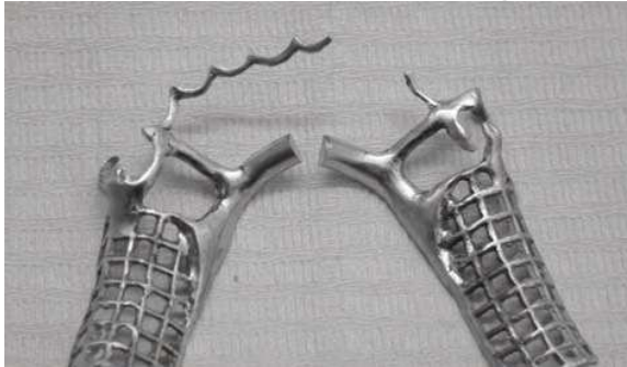
a. Cracked continuous bar & lingual bar.
