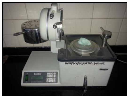
Fig.4: Fabricate a Biostar vinyl base on the cast
