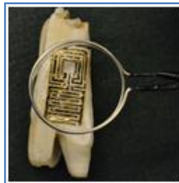
Fig. No. 2: On a cow's tooth, the sensor can detect bacteria and send a signal to a nearby receiver.
