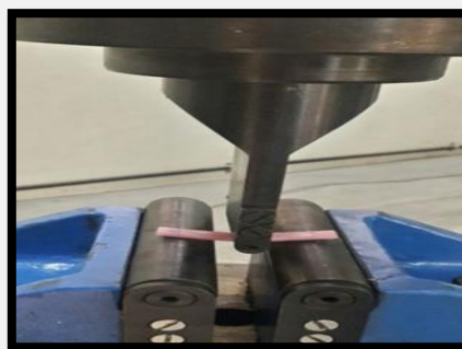
Figure 6. Specimen Placed under Load in 'Universal Testing Machine'
